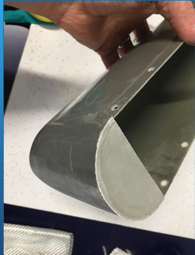
Fillet inserted & glued in place with epoxy
